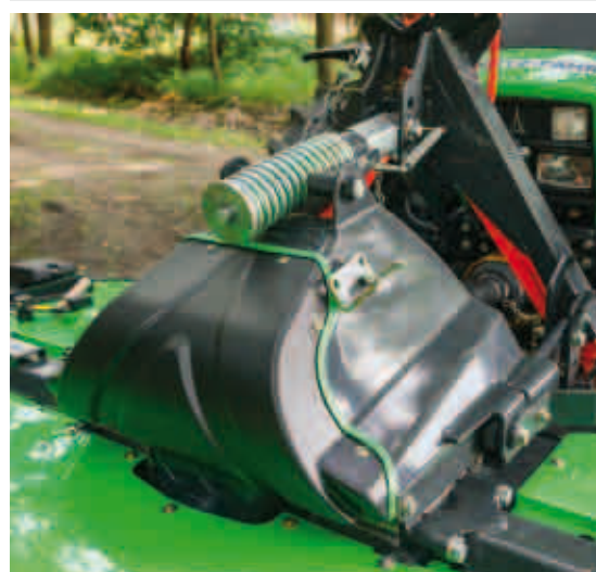
PENDEFLEX pendulum headstock
