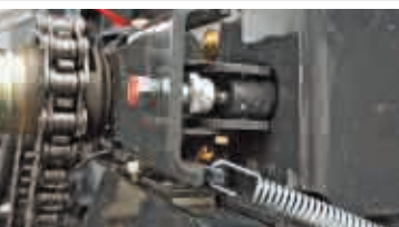
The standard hydraulic rotor clutch can be operated from the tractorcab
