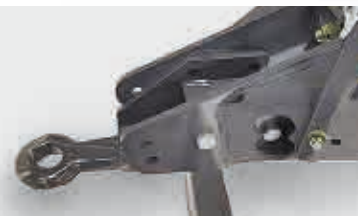
A reversible drawbar provides simple, flexible top or bottom attachment
