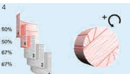
The bale is covered with 3 layers and 67% overlap
