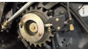
The standard, automatic chain oiling system allows individual adjustment to the amount of oil on each chain
