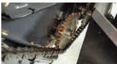
The simple driveline, with heavyduty 1 1/4" chains, is designed for minimum maintenance in the toughest conditions
