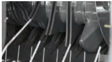
Integral Rotor Technology ensures even, force-fed intake
