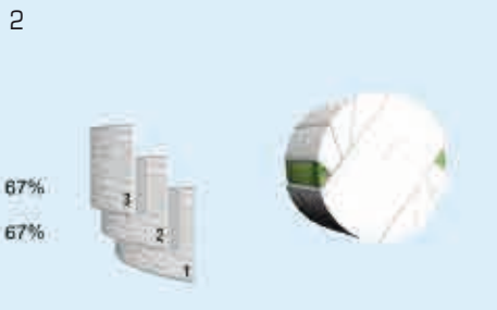
The bale is covered with 3 layers and 67% overlap
