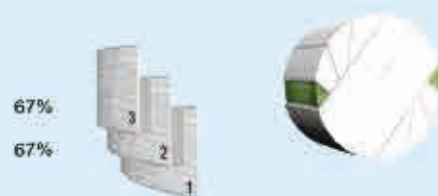
The bale is covered with 3 layers and 67% overlap
